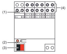
Figure 1: Device components
