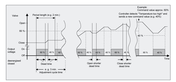
Figure 12: Ideal course of the valve stroke for a cycle time < Adjustment cycle time
