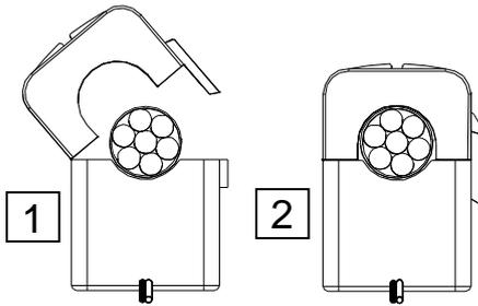
**⚠ Important:** Secondary side cables must be connected to KES Plus (keeping polarity) before closing the clamp to the primary side cable.
