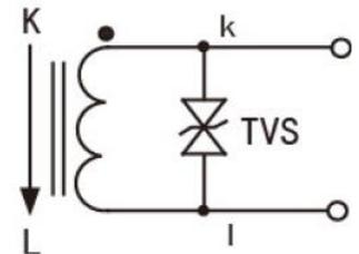
**Figure 2.** Current Transformer Schematic
